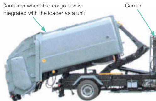
Refuse collection vehicle with an attachable and detachable body
