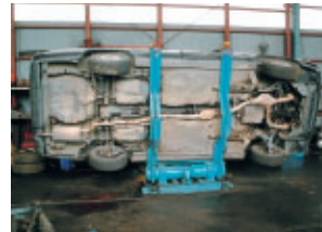
Parts can be removed easily and effectively by tilting the ELV.
