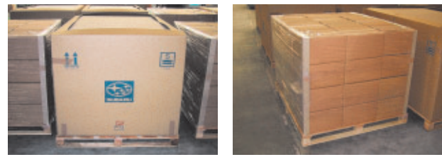
Before improvement (cardboard packaging) After improvement (stretched film packaging)
