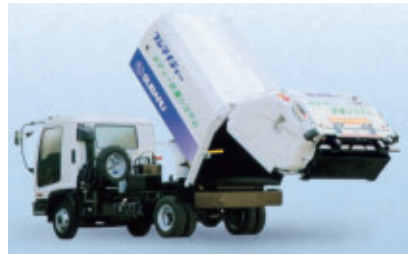
Introduction of the automatic body weighing system to the dumping discharging style refuse collection vehicle first in Japan
