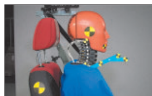
The latest whiplash measurement tool, a human dummy
