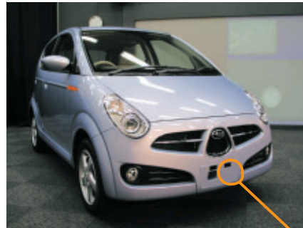
Now the material type can be seen without dismantling the bumpers. (Subaru R2)
