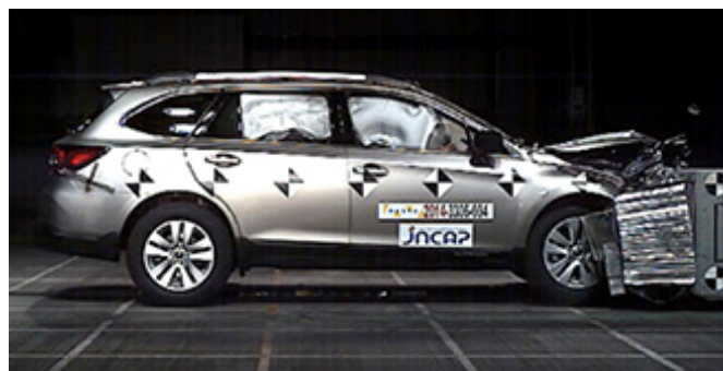
Image of Legacy Outback JNCAP Frontal Offset Crash Test Photo courtesy of the National Agency for Automotive Safety & Victim' s Aid (NASVA)
