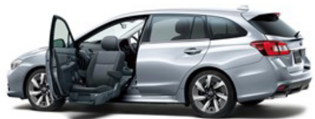
Levorg TRANSCARE Wing Seat (Lift type)
