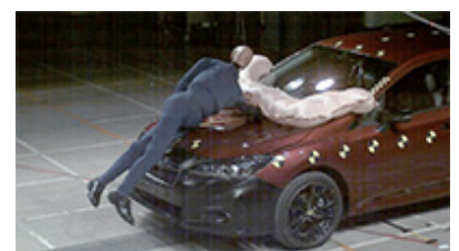
Crash test using a car fitted with the first pedestrian protection airbag in a Japanese-produced vehicle
