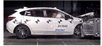
Image of Impreza JNCAP Frontal Offset Crash Test
