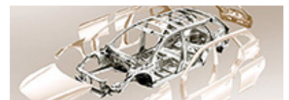
Legacy’s lightweight body that achieved both weight reduction and strength
