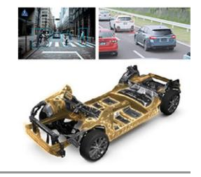
In 2017, Subaru introduced an updated version of EyeSight that features the new driving Assist function. This extends the minimum speed at which EyeSight's Lane Keep Assist function operates from 60 km/h to 0 km/h. It also adds automated steering that follows the preceding vehicle in the same lane, teamed with Adaptive Cruise Control to assist drivers with automated control of acceleration, braking, and steering on expressways, greatly reducing driver burden.
