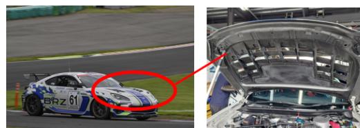
Lightweight bonnet hood using recycled carbon fiber
