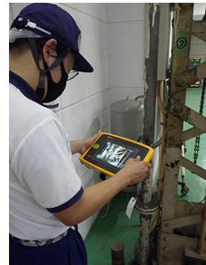
Air leak investigation
