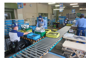
The height of automatic door switches and work stations is set at a level that is convenient for those using wheelchairs
