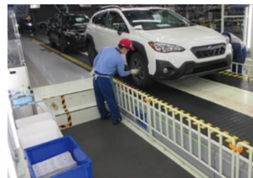
processes at undercarriage using a lowered floor to reduce the burden on inspectors, and a wide conveyor that moves across the entire floor so that inspectors can concentrate on inspection without walking from place to place. These standard inspection lines offer flexibility and expandability to accommodate BEV\* production, and will be passed on to the dedicated BEV line at the Oizumi Plant, which is currently under construction.
