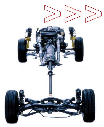
A full-time 4WD system, horizontally opposed engine and symmetrical layout with a low center of gravity are core technologies that underpin Subaru's success.
