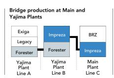
Bridge production of the Impreza and Forester models serves as a kind of control valve, allowing the lines to respond flexibly to demand for each model and maximize the utilization of production capacity.
