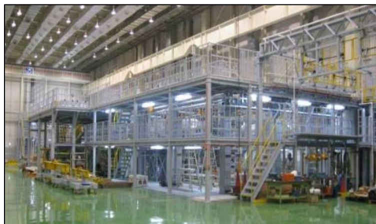
The 3 rd Production Line for the Boeing 787 Center Wing Box Assembly at Handa Plant
