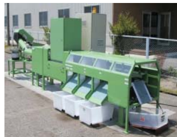
Bottle Hunter (Automatic color sorting equipment for glass and PET bottles)
