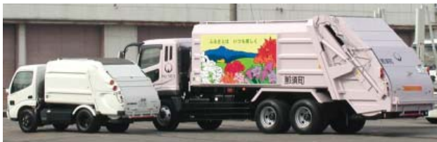
General 4 m 3 refuse collection vehicle (left) and large 20m 3 press-style refuse vehicle (right)
