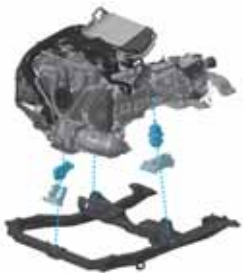
Cradle structure: newly designed as a powertrain mounting system
