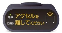
Device to prevent unintended acceleration from pedal misapplication: in-vehicle indicator (when activated; conceptual illustration)
